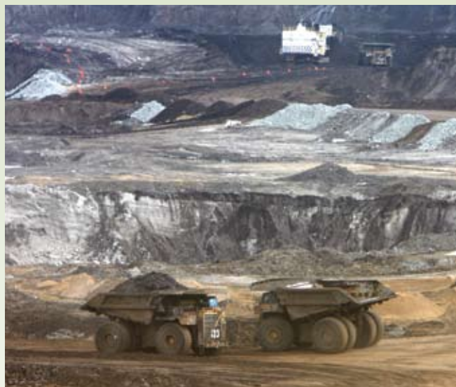
Figure 15-13 Huge trucks and machines extract earth from an open pit mine near Fort McMurray. Hot water is then used to separate the oil from the sand.
